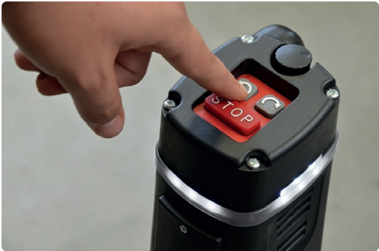
Counterclockwise (CCW) rotation User-friendly control of tapping tool retract
