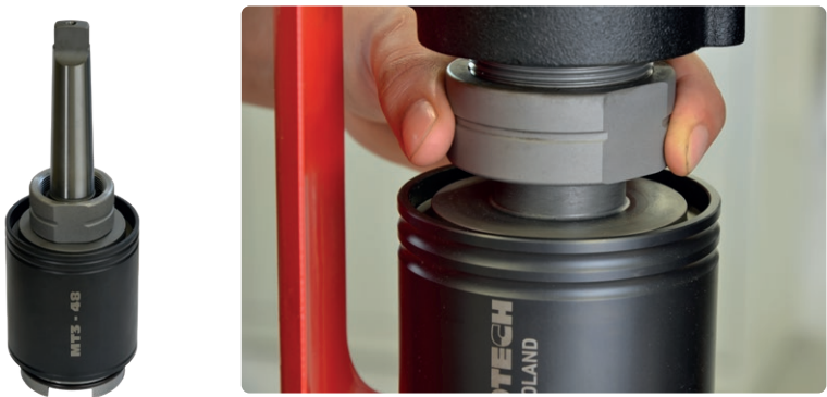
Tapping chuck equipped with securing nut protects tapping tool against pull out
