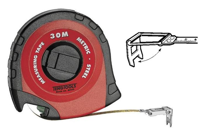
**Teng Tools** Steel measuring tape with nylon coating and anti-reflection surface. 10 mm tape width. Graduated in mm and inch. High impact plastic case with rubber grips on the sides. True zero hook for internal and external measurement.
