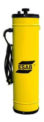
The PSE are light and handy dry-storage containers for electrodes. It is easy to carry and has a manual thermostat with a high range in storage temperature. The heating element runs from the top to the bottom and the top is fully insulated.
