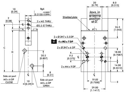
NOTE: Jaws have to be designed for a 0° gripping position (parallel jaws). Jaws will close 1.5° past parallel. To limit shocks at the end of an opening or closing stroke, it is highly recommended to design jaws with minimal inertia (as light and short as possible). Flow Controls make it possible to reduce the rotation speed and are highly recommended.
