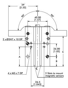
NOTE: Jaws have to be designed for a 0° gripping position (parallel jaws).Jaws will close 1.5° past parallel. To limit shocks at the end of an opening or closing stroke, it is highly recommended to design jaws with minimal inertia (as light and short as possible). Flow Controls make it possible to reduce the rotation speed and are highly recommended.
