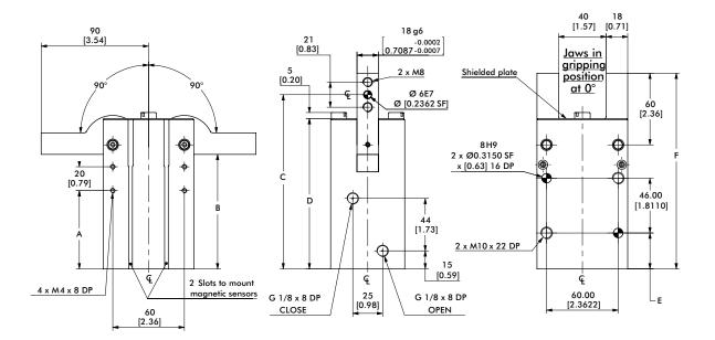
NOTE: Jaws have to be designed for a 0° gripping position (parallel jaws).Jaws will close 1.5° past parallel. To limit shocks at the end of an opening or closing stroke, it is highly recommended to design jaws with minimal inertia (as light and short as possible). Flow Controls make it possible to reduce the rotation speed and are highly recommended.
