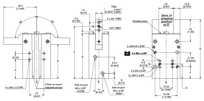
NOTE: Jaws have to be designed for a 0° gripping position (parallel jaws).Jaws will close 1.5° past parallel. To limit shocks at the end of an opening or closing stroke, it is highly recommended to design jaws with minimal inertia (as light and short as possible). Flow Controls make it possible to reduce the rotation speed and are highly recommended.
