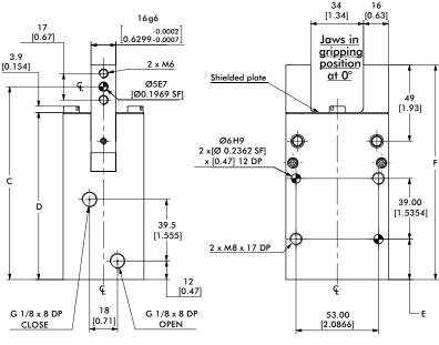
NOTE: Jaws have to be designed for a  $0^{\circ}$  gripping position (parallel jaws). Jaws will close 1.5° past parallel. To limit shocks at the end of an opening or closing stroke, it is highly recommended to design jaws with minimal inertia (as light and short as possible). Flow Controls make it possible to reduce the rotation speed and are highly recommended.
