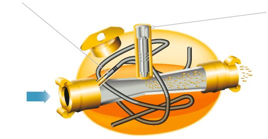
Chicago Pneumatic's lubricators use the ejector principle to create controlled lubrication. The pick-up is intricately bent to the assure oil supply regardless of the lubricator's position.
